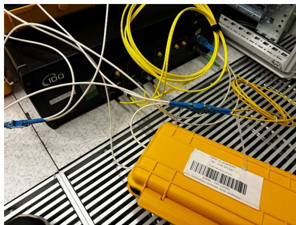
Figure 25: Fibre launch leads with splitter
