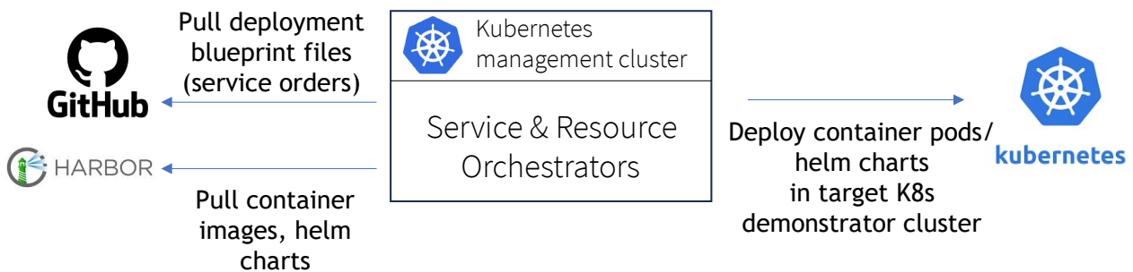
Figure 5-2: Reference CD pipeline with Service Orchestration.
