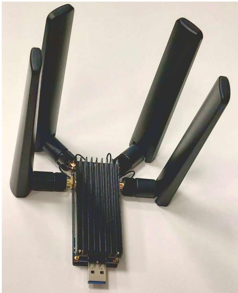
Figure 25: USB Dongle with Quectel 5G Module
