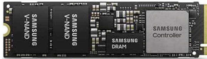
Figure 30: Samsung PM9A1 MZVL2512HCJQ - SSD - 512 GB - PCIe 4.0 x4 (NVMe)
