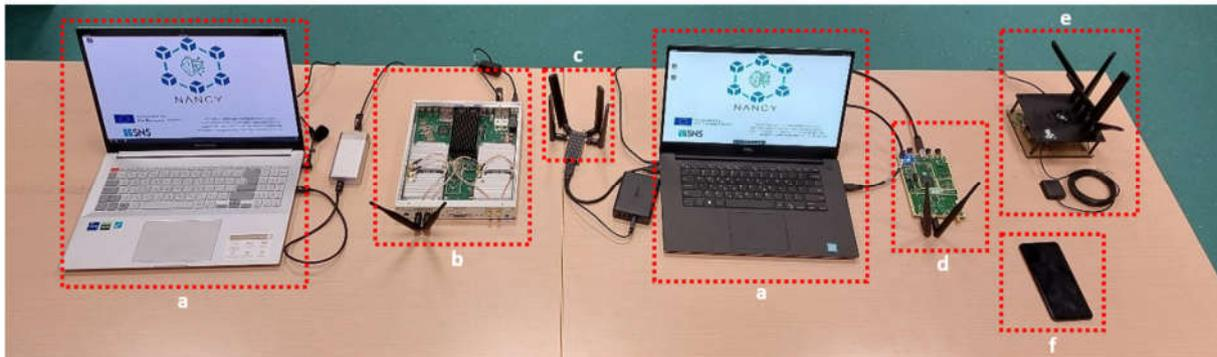
Figure 6: Greek in-lab testbed hardware. a) High performance laptops, b) USRP X310, c) USB Dongle with Quectel 5G Module, d) USRP B210, e) SIM8200A-M2 5G Hat, f) Mobile Phone
