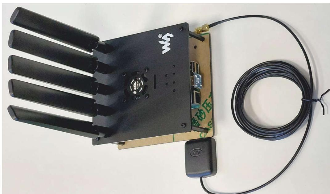
Figure 26: Waveshare SIM8200A-M2 5G Hat for RaspberryPi
