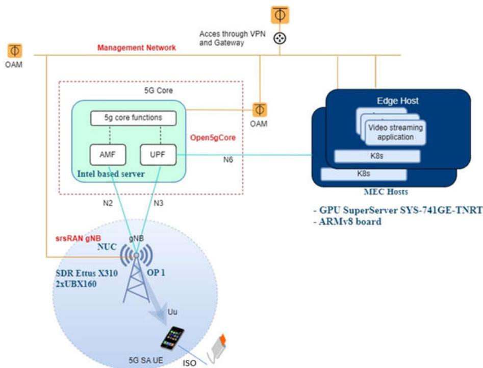
Figure 12: Italian in-lab testbed topology and configuration
