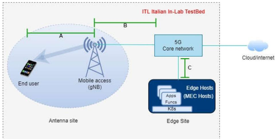
Figure 13: Italian In-lab testbed: network segments for measurements - A, B and C
