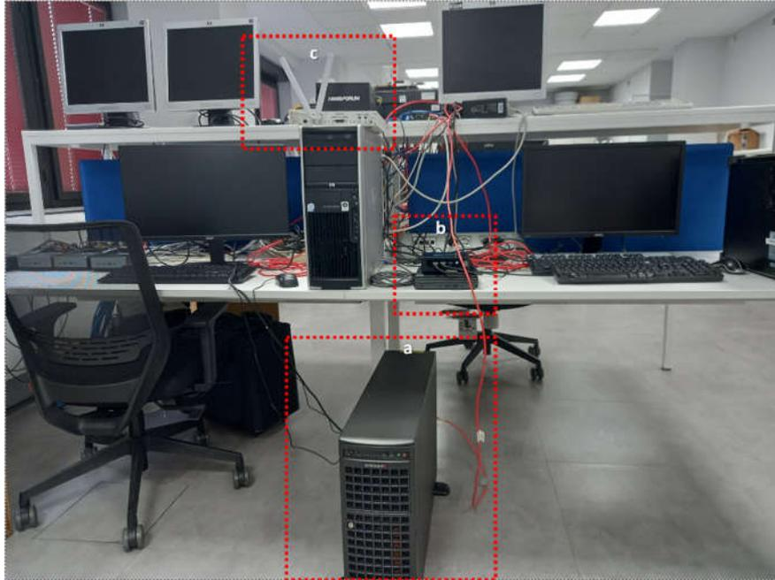
Figure 9: NANCY's Italian in-lab testbed - picture 1: a) GPU SuperServer SYS-741GE-TNRT + 2 GPU NVIDIA A40, b) Intel® NUC, c) USRP X310
