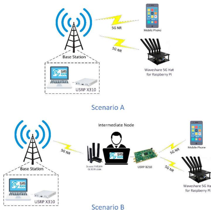
Figure 8: Experimental Activities in the Greek In-lab testbed
