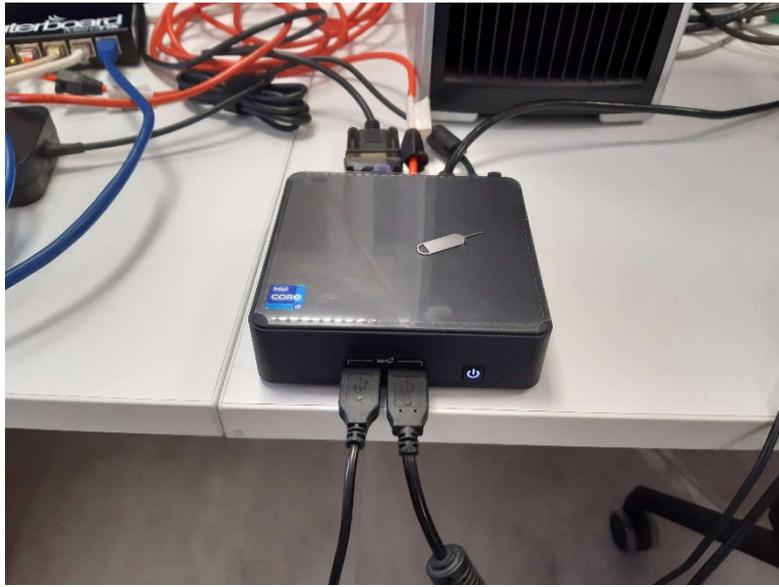
Figure 24: Intel Next Unit of Computing (NUC) 12 Pro Kit - NUC12WSKI7 in the Italian testbed
